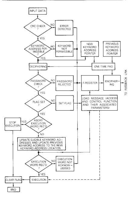
Figure 4. Flow Chart for the Recipient's Authentication Subsystem
