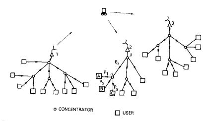
Figure 4. A Typical Architecture of Digital Communications Networks with Levels of Hierarchy
