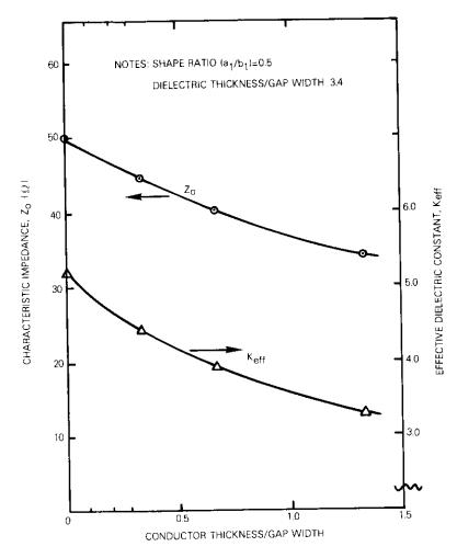
Figure 3. Line Parameter Dependence on Conducting Strip Thickness
