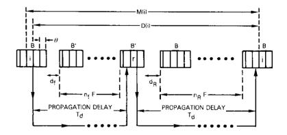
Figure 7. Illustration of Effective Propagation Delay D(i) in a TDM System in the Case of Multiple Superframe per Burst Operation With Acknowledgments Attached to Superframes
