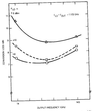
Figure 26. Measured Performance of the MIC Up-Converting Mixer
