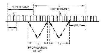
Figure 5. Representation of TDM System Case of Multiple Bursts per Superframe Operation With Short Acknowledgments
