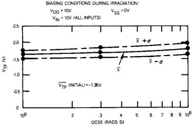
b. THRESHOLD VOLTAGE OF P-CHANNEL DEVICES, VTP (INCLUDES ALL THREE LEVELS OF INTEGRATION; SOLID LINE INDICATES MEAN VALUE AND DASHED LINES INDICATE ONE STANDARD DEVIATION)
