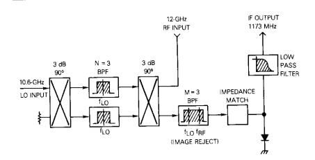
Figure 12. MIC Mixer Block Diagram
