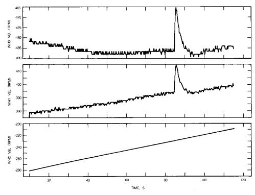
Figure 10. Wheel Failure with Four Reaction Wheels (Example 1) (sheet 2 of 3)
