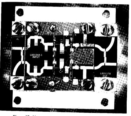
Figure 27. Photograph of 14-GHz Balanced FET Amplifier
