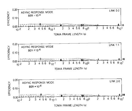
Figure 10. Net Throughput Efficiency for One-Way Data Flow and a Preamble Plus Guard Time of 50  $\mu$ s (BER = 10<sup>-4</sup>; curves represent different superframe sizes in K bytes)
