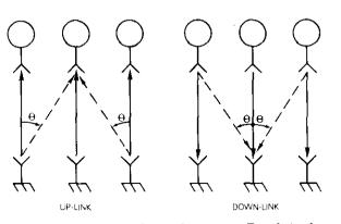
Figure 6a. Two Interfering Sources at Equal Angles
