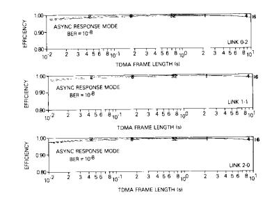
Figure 12. Net Throughput Efficiency for One-Way Data Flow and a Preamble Plus Guard Time of 50  $\mu$ s (BER = 10<sup>-8</sup>; curves represent different superframe sizes in K bytes)
