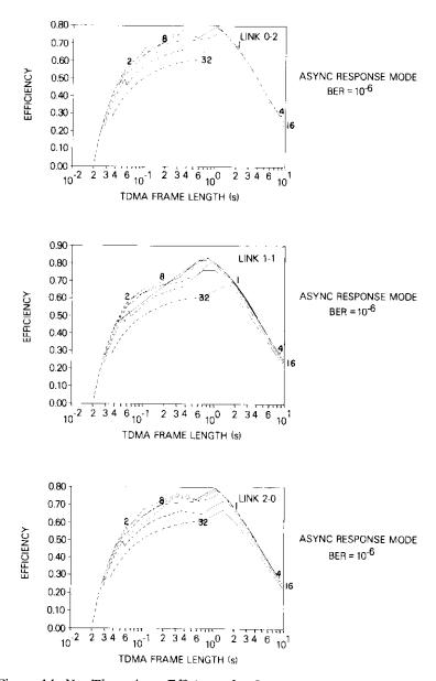
Figure 14. Net Throughput Efficiency for One-Way Data Flow and a Preamble Plus Guard Time of 5 ms ( $BER = 10^{-6}$ ; curves represent different superframe sizes in K bytes)
