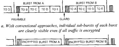
b. With multiple-destination cryptosystems, the entire burst appears as a single entity
