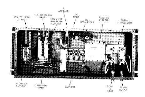
Figure 5. Photograph of Down-Converter
