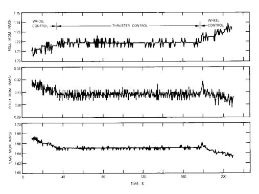
Figure 8. Stationkeeping by Applying a Weight on the Platform (thruster control) (sheet 3 of 3)
