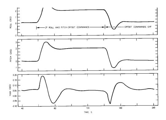
Figure 5. Transient Response for Four Reaction Wheels
