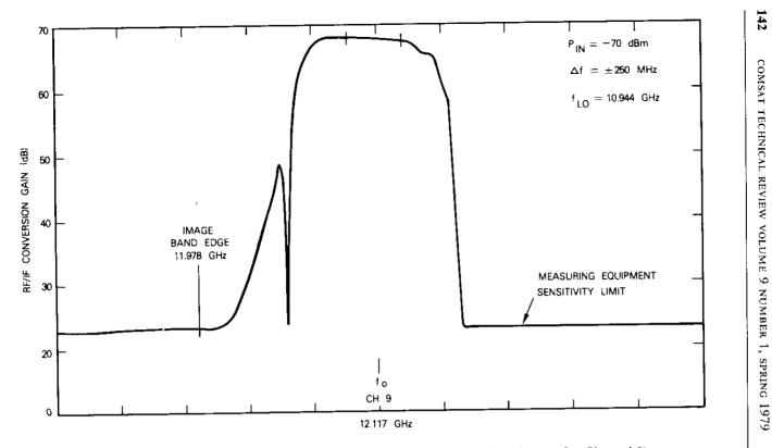
Figure 19. Down-Converter Conversion Gain vs Input Frequency (LO Chosen for Channel 9)
