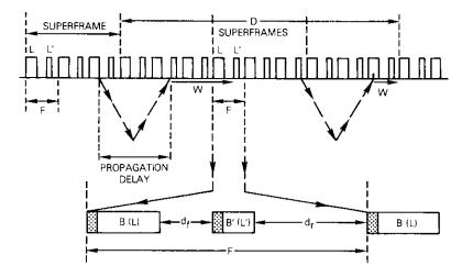
Figure 4. Representation of TDM System Case of Multiple Bursts per Superframe Operation With Acknowledgments Piggybacked on Data
