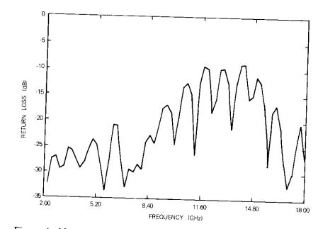
Figure 4. Measured Return Loss of a 5.08-cm CPW Line with SMA Transitions (Termination is an SMA load)
