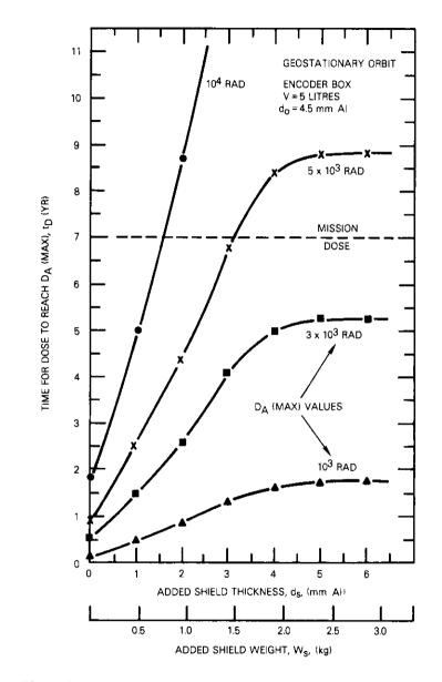
Figure 2. Survival of CMOS Circuits in a Particular Location of a Communications Satellite (from Reference 3)
