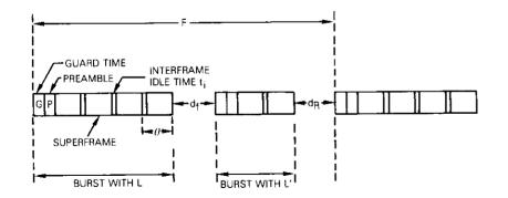
Figure 6. Representation of TDM System Case of Multiple Superframes per Burst Operation and Burst Structure
