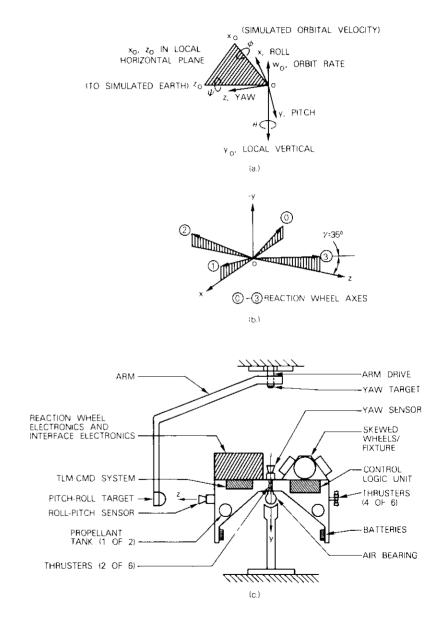
Figure 3. Control System on Test Facility
