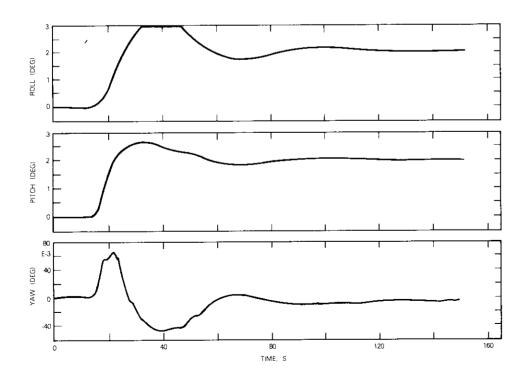
Figure 6. Transient Response with Uncorrected Failure of Wheel 0 (offset commands)
