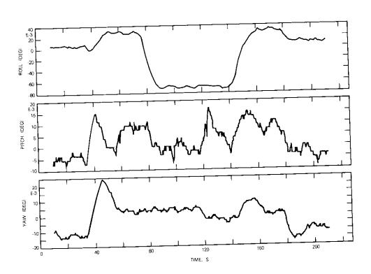
Figure 8. Stationkeeping by Applying a Weight on the Platform (thruster control) (sheet 1 of 3)
