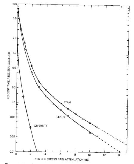
Figure 3. Cumulative Distributions of 11.6-GHz Excess Rain Attenuation Observed at Etam and Lenox from October 25, 1977, to October 24, 1978, and the Distribution Observed for Path Diversity Between These Sites During the Same Period (Straight-line extrapolations for the single-site distributions for attenuations above 11 dB are designated by the dashed lines.)
