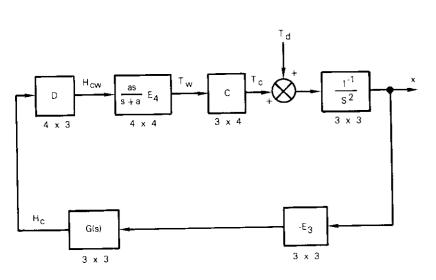
Figure 4. Block Diagram of the Simplified Control System
