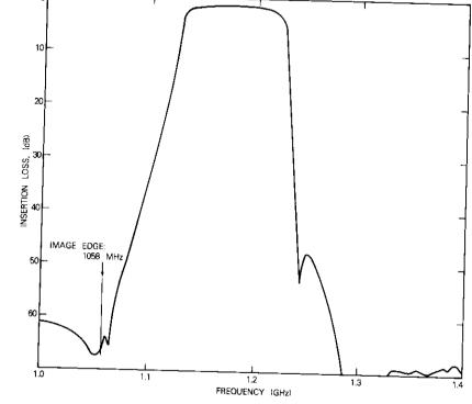
Figure 17. Measured Insertion Loss of IF Filter with N = 7,  $\delta = 0.1 \, dB$ ,  $BW = 120 \, MHz$ ,  $f_o = 1173 \, MHz$
