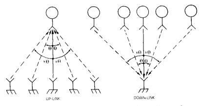
Figure 6b. Two Interfering Sources at Angle  $\theta$  and Two at  $k\theta$
