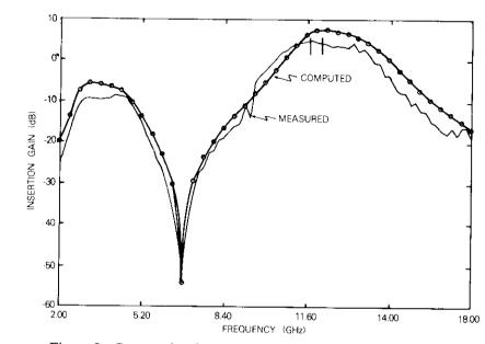
Figure 9. Computed and Measured Response of 1-Stage CPW FET Amplifier
