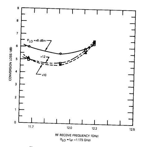
Figure 14. Measured MIC Mixer Performance
