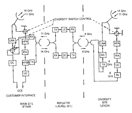
Figure 5. U.S. Standard C Earth Station Block Diagram Showing Diversity Interconnection Link (Etam-Lenox, W. Va.)
