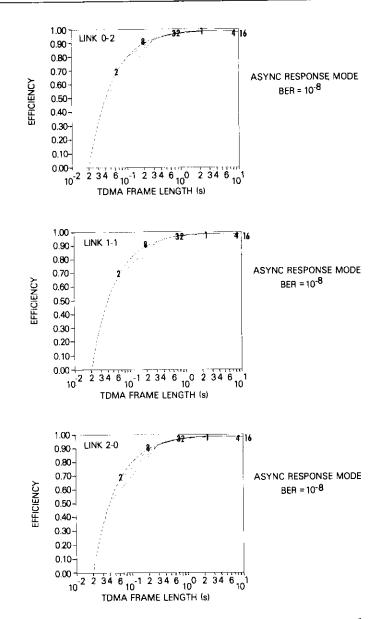
Figure 15. Net Throughput Efficiency for One-Way Data Flow and a Preamble Plus Guard Time of 5 ms ( $BER = 10^{-8}$ ; curves represent different superframe sizes in K bytes)
