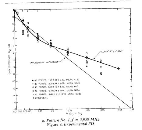
All of the curves fall above the exponential curve for probabilities greater than 50 percent, indicating that the pattern is less likely to have low values of gain than would be predicted by the exponential PDF. This may be attributable to the low recorded signal level corresponding to noise level.
