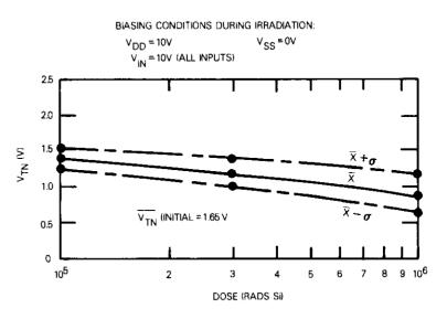
a. THRESHOLD VOLTAGE OF N-CHANNEL DEVICES, V<sub>TN</sub> (INCLUDES ALL THREE LEVELS OF INTEGRATION; SOLID LINE INDICATES MEAN VALUE AND DASHED LINES INDICATE ONE STANDARD DEVIATION)
