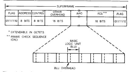
Figure 1. Superframe Format and BLU Structure (Basic logic units may all be for the same destination or for different destinations.)
