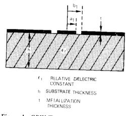
Figure 1. CPW Transmission-line Definitions
