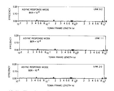
Figure 16. Net Throughput Efficiency for Piggybacked Acknowledgments With All Nodes Transmitting and a Preamble Plus Guard Time of 50  $\mu$ s (BER = 10<sup>-4</sup>; curves represent different superframe sizes in K bytes)
