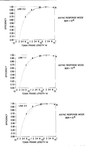
Figure 20. Net Throughput Efficiency for Piggybacked Acknowledgments With All Nodes Transmitting and a Preamble Plus Guard Time of 5 ms (BER =  $10^{-6}$ ; curves represent different superframe sizes in K bytes)
