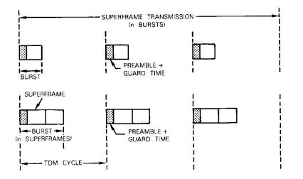
Figure 3. Illustration of the Case of Multiple Bursts per Superframe and the Case of Multiple Superframes per Burst
