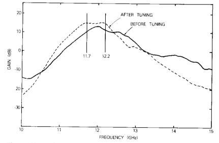
Figure 10. Performance of Two Single-Stage CPW FET Amplifiers Cascaded in a Single Support Structure
