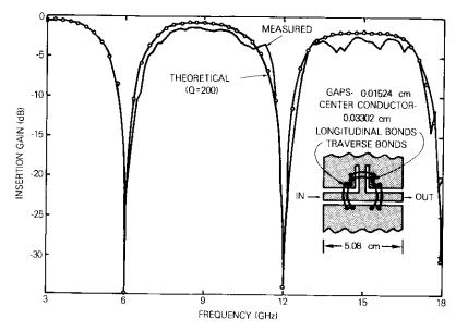
Figure 6. Measured and Theoretical Transmission Loss for a CPW Shunt Shorted Stub on a 5.08-cm Through Line
