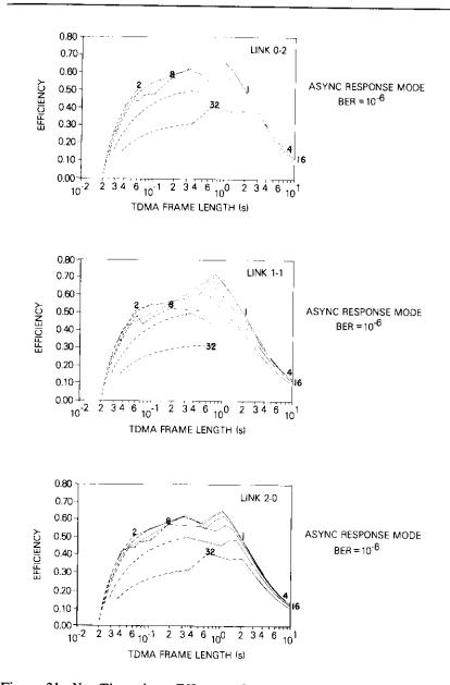
Figure 21. Net Throughput Efficiency for Piggybacked Acknowledgments With All Nodes Transmitting and a Preamble Plus Guard Time of 5 ms (BER =  $10^{-8}$ ; curves represent different superframe sizes in K bytes)
