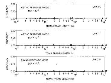
Figure 19. Net Throughput Efficiency for Piggybacked Acknowledgments With All Nodes Transmitting and a Preamble Plus Guard Time of 5 ms (BER =  $10^{-4}$ ; curves represent different superframe sizes in K bytes)
