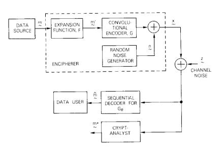
Figure 2. Block Diagram of the Proposed Cryptosystem
