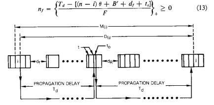
Figure 8. Illustration of Effective Propagation Delay D(i) in a TDM System in the Case of Multiple Superframe per Burst Operation and One-Way Data Flow
