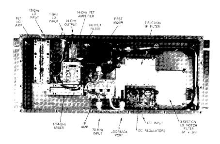
Figure 23. Photograph of MIC Up-Converter
