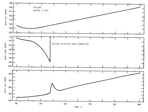
Figure 11. Wheel Failure with Four Reaction Wheels (Example 2) (sheet 2 of 2)
