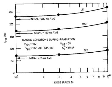
d. PROPAGATION DELAY, TFD, FOR THREE LEVELS OF INTEGRATION
