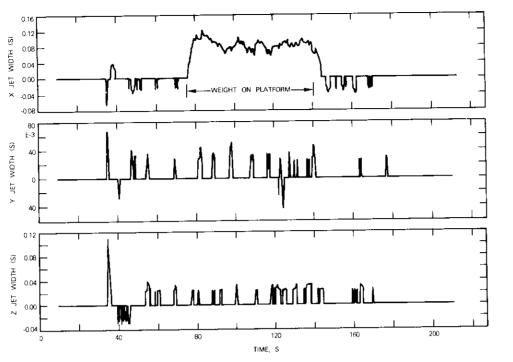
Figure 8. Stationkeeping by Applying a Weight on the Platform (thruster control) (sheet 2 of 3)
