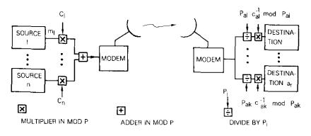
Figure 5. The Implementation of the Proposed Multiple-Destination Cryptosystem for Broadcast Networks
