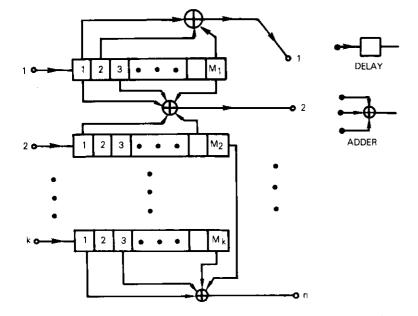
Figure 3. k-Input, n-Output Feed Forward Linear Sequential Circuit (FFLSC)
