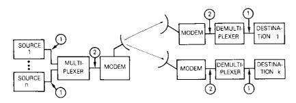
Figure 1. A Typical Broadcast Network and Two Commonly Used Approaches to Provide Communications Security
